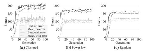
Fig. 5 Best and mean fitness, measured as foraging efficiency (resources collected per hour, per swarm) for simulated swarms foraging on **a** clustered, **b** power law, and **c** random resource distributions with and without real-world sensor error. Results are for 100 replicates
