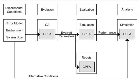
**Fig. 2** We use a GA to **evolve** a foraging strategy (CPFA parameter set) that maximizes resource collection for specified classes of error model, environment, and swarm size. We then *evaluate* the foraging strategy in multiple experiments with simulated and physical robots and record how many resources were collected. We repeat this for different error models, environments, and swarm sizes. We *analyze* flexibility by evolving parameters for one condition and evaluating them in another
