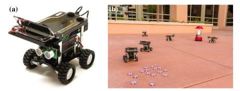
Fig. 1 a An iAnt robot. b A swarm of iAnt robots foraging for resources around a central illuminated beacon
