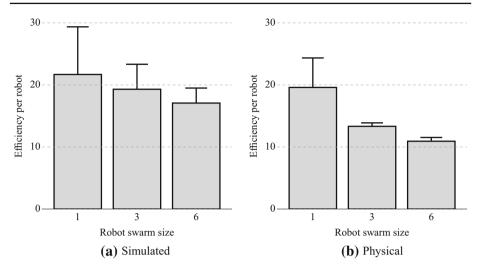
**Fig. 10** Foraging efficiency (resources collected per hour, per robot) of *1*, *3*, and *6* robots foraging on a power law distribution for **a** swarms in a simulation that includes sensor error and **b** physical swarms. All results are statistically different (p < 0.001)
