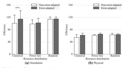
**Fig. 6** Foraging efficiency (resources collected per hour, per swarm) using error-adapted and non-erroradapted parameters for **a** 6 robots foraging in a simulation that includes sensor error and **b** 6 physical robots. *Asterisks* indicate a statistically significant difference (p < 0.001)
