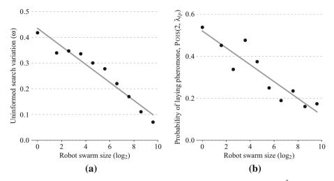
**Fig. 12** a Swarm size versus best evolved uninformed search variation ( $\omega$ ) (slope = -0.035,  $R^2 = 0.94$ , p < 0.001) (see Fig. 14 in supplementary material for statistical distribution). **b** Swarm size versus best evolved probability of laying pheromone when two resources are found in the resource neighborhood (Eq. 4:  $k \leftarrow 2$ ,  $\lambda \leftarrow \lambda_{lp}$ ) (slope = -0.040,  $R^2 = 0.84$ , p < 0.001) (see Fig. 14, supplementary material)
