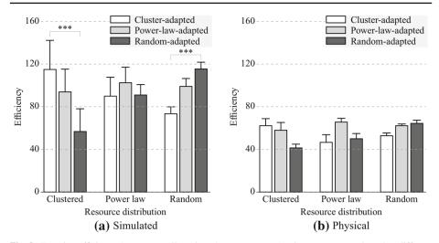
**Fig. 8** Foraging efficiency (resources collected per hour, per swarm) using parameters adapted to different resource distributions for **a** 6 robots foraging in a simulation that includes sensor error and **b** 6 physical robots. *Asterisks* indicate a statistically significant difference (p < 0.001)
